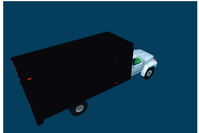
Figure 9: Final HVE model of incident roofing truck
